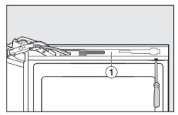
Prise open panel ① from the soft-close mechanism by inserting a flat-bladed screwdriver into the gap from above and easing it off bit by bit.
